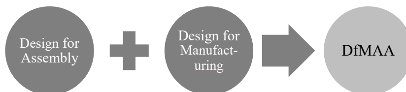
Figure 1-1: Conceptual relationship between design for manufacture and design for assembly in DfMA
